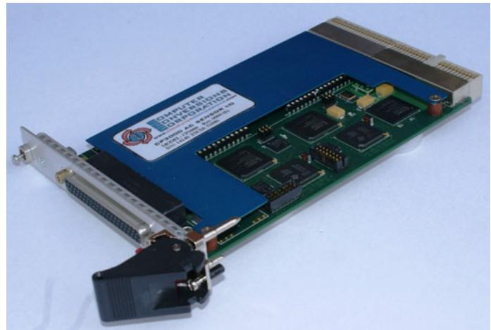
The input channel Syncro / Resolver Input Channels are supplied with internal mirror I/O that is used to exercise input circuitry functionality to provide continuous and comprehensive self testing that operates quietly in the background without any user programming or intervention required.
