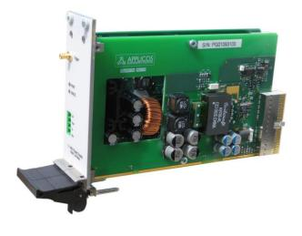
The PS48401 is a Programmable DC Power supply in a 2-slot PXI / cPCI form factor. Featuring a fully isolated output capable of providing 0-48VDC / 2A / 40W. It offers a programmable current limit and the ability to measure the output voltage and current under software or trigger control.
