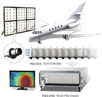
A highly efficient and precise test and measurement solution based on PXI Express (PXIe) architecture, with multiple channels and fully integrated synchronization, can connect with sensors to measure various parameters to streamline system installation.
