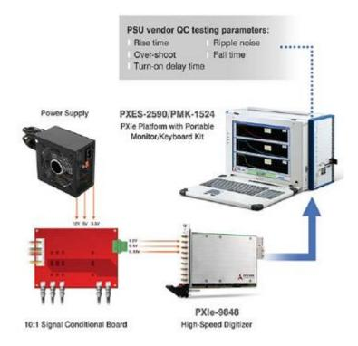
By taking advantage of the inherent modularity of the PXI interface, however, power supply unit test systems can quickly adapt to changing measurement requirements with increases in performance and speed of units to be tested.
