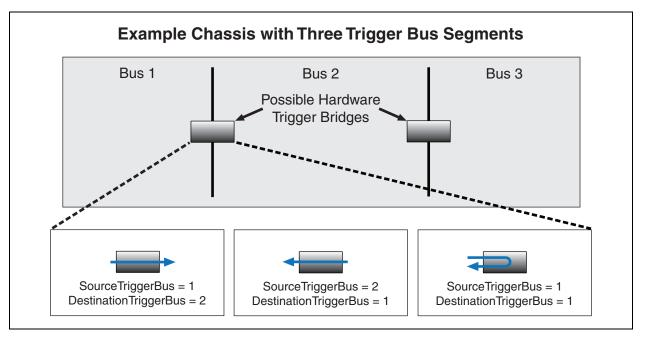
**Figure 2-1.** A hardware trigger bridge may have multiple software representations in the chassis description file, supporting one or more of the capabilities shown in this figure. It must have a separate trigger bridge descriptor for each software representation.
